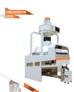
Combi separator machines have one machine frame, one common vibrator drive, one machine housing for three operations. Combi separator machines have compact and space saving design and also two machine in one
