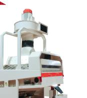
Combi separator machines have one machine frame, one common vibrator drive, one machine housing for three operations. Combi separator machines have compact and space saving design and also two machine in one
