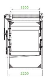
It is produced for cleaning of multiple oilseeds, like white cotton seed, sun flower kernels, soybeans, ground nuts...etc., only the perforated screens to be changed according to the processed seed.
