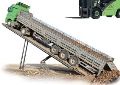
Truck Tipping Platform
