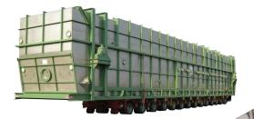
Bucket Extractor: is now the most advanced alternative to all existing extractors. The continuous series of buckets moving in roller rails, transport the oilseed over the upper and lower cylindrical buffer with agitator, level control and speed controlled dosing screws. The extractor has variable speed drive and several miscella feed tubes. Capacities 200; 500; 700; 1250 t/24 h prepressed sunflower cake.
