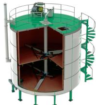
Fertilizer dryer consists of 2 decks. Product received to machine are discharged in 7-15 days. Available rotor for mixing motion. Levers on rotor are injected air to fertilizer and provided continue mixing. Injected hot air is ensured to reduce fertilizer fermentation time. When product is finished the motion in first section, it is received to second section by passing gate.
