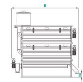
It is developed to sort the rice according to its width/thickness. We use this machine to separate raw seed, milky piece, broken and rice from each other. To make different kind of sorting, you need to change the sieve drum.
