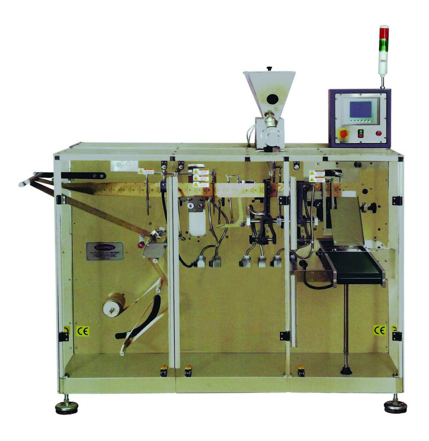
YODM/180 Sachet Packaging Machinery is a full automatic machinery with PLC control which designed for producing 3 or 4 side sealed packs. Filling System for the machine produces as Volumetric, Auger (Screw) and/or Liquid filling system according to the products to be packed Filling volume of the machine is between 10-200 ml The main usage area for this machine is to pack products like spices, sauces, soup mix, tea, coffee, cream, ketchup, mayonnaise, yeast powder, shampoo, etc.
