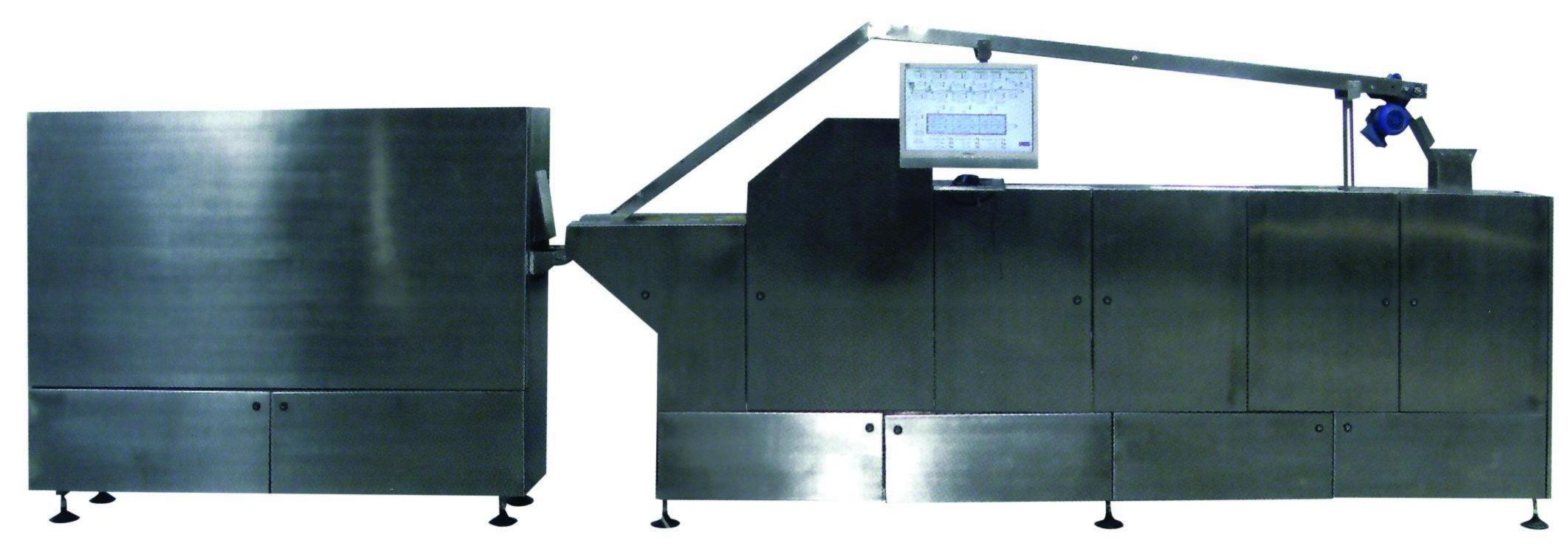
DESIGNED FOR BISCUIT PRODUCTION TEST WORKS. TEST CAN BE DONE WITH APPROX 3-4 KG DOUGH. SOFT, HARD AND WITH ADDITIONAL MACHINES TESTING CAN BE DONE WITH ALL KINDS OF BISCUITS. SAMPLE TYPE MOLD WITH ONE SINGLE ROW WITHOUT WASTE DOUGH BISCUITS TO TEST. PREVENTS WASTE DOUGH BY FORMING SAMPLE BISCUITS WITH ONE ROW SHAPE.
